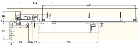
Fixing position: Where intumescents are to be fitted, 1 mm must be added to all dimensions (see fitting instructions)
