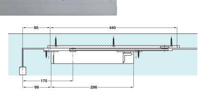
Fixing position: Where intumescents are to be fitted, 1 mm must be added to all dimensions (see fitting instructions)
