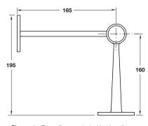
Please note: These railing supports should not be wall mounted for use as handrail support. These supports should only be base mounted as shown
