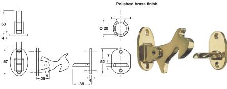
Overall dimension when fitted = 89 mm
