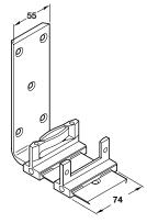
Note: For extra thick single doors use B, cut base plate back to required size and discard cavity panel connector
