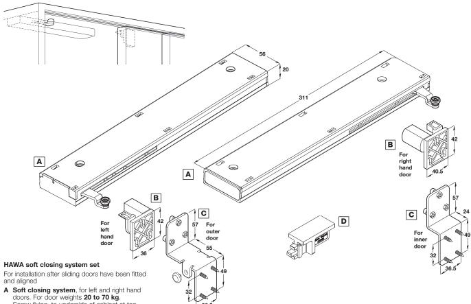
A Soft closing system, for left and right hand doors. For door weights 20 to 70 kg. Screw fixing, to underside of cabinet at top. Light grey plastic housing, zinc plated steel arm mechanism with white nylon roller
