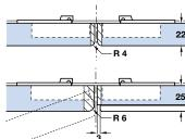
For door thickness 20+ mm, edges must be radiused
