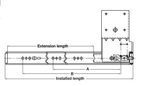
Installed length = Minimum carcase depth required to install fitting Extension length = Maximum door width that can be withdrawn inside the carcase
