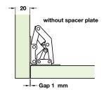
Examples of corner gap measurements for single sided overlay door mountings
