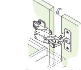
Zero protrusion for application with inset drawers. With 00 cranking and 00 height of mounting plate the door is flush with the cabinet at 90°
