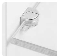
Pressing down on the tightening element fixes the glass shelf in position. The shelf support prevents it from tipping as well as being unintentionally lifted and removed.
