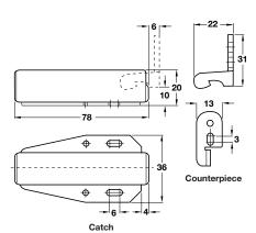
A guide is supplied to centre the drill-hole for the slot in the counterpiece. It is placed in the catch housing and will locate the drilling centre when the door is pressed against it.
