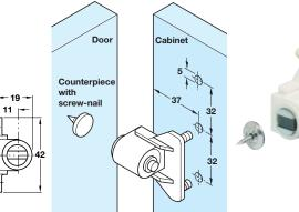
Drilling and mounting diagram
