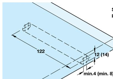
Dimensions in brackets are for shelf thickness 22 mm using 14 mm size shelf support
