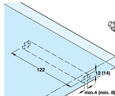
Dimensions in brackets are for shelf thickness 22 mm using 14 mm size shelf support
