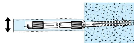
Adjustable in height and inclination
