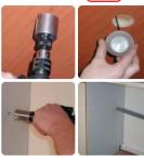
Cable outlet cutters can be used for a variety of applications where cables or pipes need to be inserted/ passed through wooden obstructions
