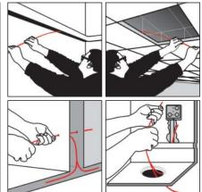
The cable guide rod set and accessories make the installation of wiring quick and simple. The range of different fibre rods and brass acessories can be used in a vast amount of configurations allowing greater flexibility and ease of use
