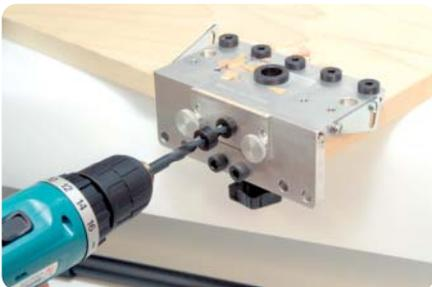
**Panel drilling** - The clamping device secures the drilling position. This allows quick drilling of hole series at a distance of 37 mm from the front edge of the carcass and 60 mm from the rear edge of the carcass. Locating pins make it easy to position the clamping device
