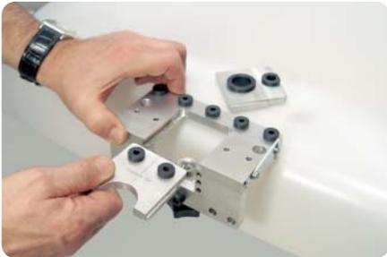
**Edge drilling** - The drill insert for edge drilling allows adjustment to 16/19/22 mm panel thickness or 15/18 mm panel thickness
