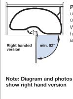
**Please note**: 92° cabinet hinges must be used, as door needs to open a minimum of 92° to allow the unit to pull out. Wide corner post must also be fitted, if D
