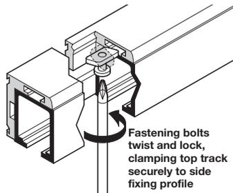
Fastening bolts twist and lock, clamping top track securely to side fixing profile
