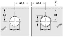
\*32 mm hole for glass door lever lock with architectural cylinder
