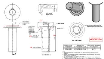
TPU OVERMOULD PROPOSED MATERIAL TO BE APPROVED BY HGT PRIOR TO MANUFACTURE
