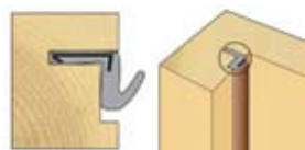
Diagrams of how Aquamac Weatherseal is fitted
